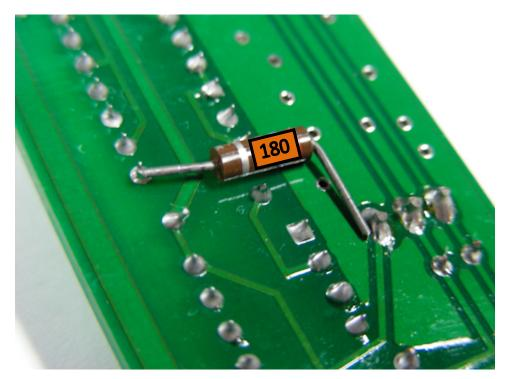
When you are satisfied with the fit, solder the resistor leads to the voltage regulator and #15 PIC pin. As an option, I recommend a piece of tape to hold the resistor in place while soldering the first lead. Remove the tape, adjust for a perfect fit one last time then solder the remaining lead.
