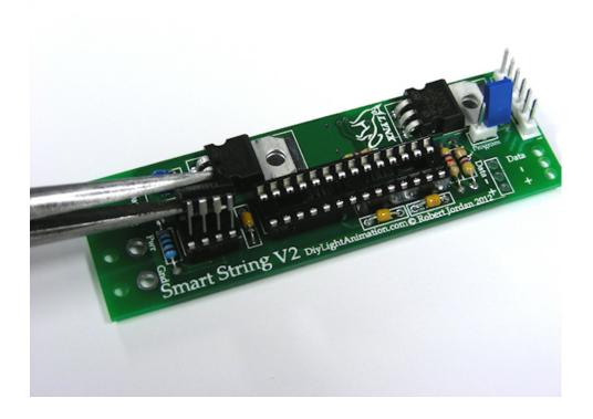
De-solder and remove the +, -, and data wires from the SSC, if attached.
