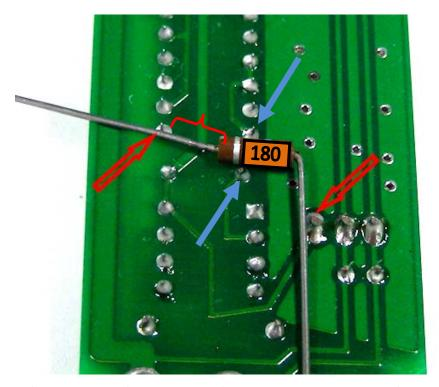
Trim the leads of the resistor to fit the spacing of the pins on the board. Trial fit this resistor several times to make sure it fits well and does not contact other near-by pins.
