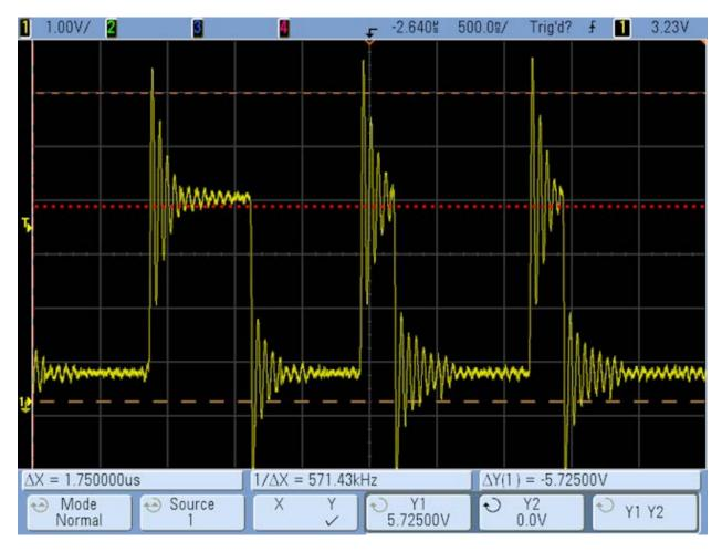
The new WARP DRIVE modification uses a different pin on the PIC chip which can fully support 5 volt output to the nodes. This returns the PIC chip to well within the published operating specs. The data signal is boosted to a solid 5 volts – which is exactly what the node expects to see and far in excess of the 3.5V minimum requirement (red dashed line).
