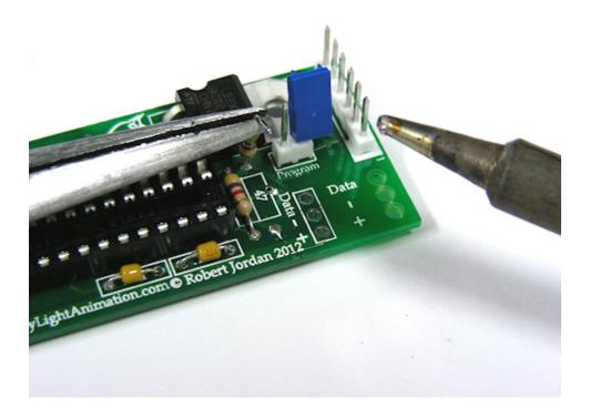
Use a small amount of solder to 'retouch' the holes left in the circuit board. They should be left with a small, clean rounded dome of solder.
