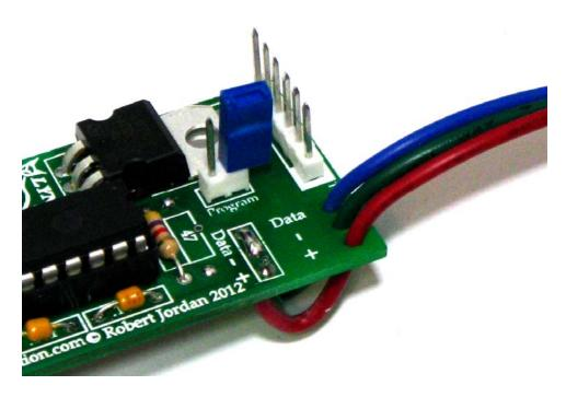
At this point, build a solder bridge from the – lead to the now empty 'data' lead hole. This will properly ground the poor old, burnt up, over driven data pins on the PIC and put them to rest once and for all. Thank you for your valiant service, rest in peace!!
